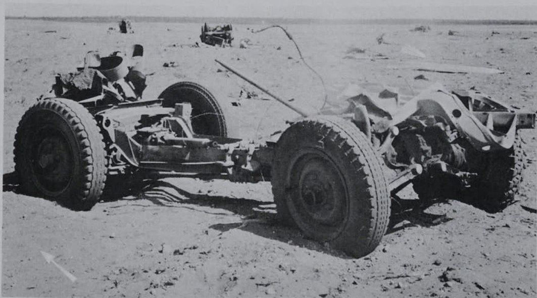
FIGURE 16. ROUND 3. VIEW OF FRONT 4 CHAMPS AFTER FIRING WITH SCATTERED DEBRIS
